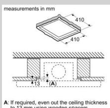
A: If required, even out the ceiling thickness to 13 mm using wooden spacers.
