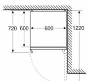
Measurements in mm
