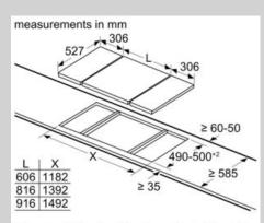
When installing two Domino units right next to a hob, two assembly kits (HEZ394301) are required.
