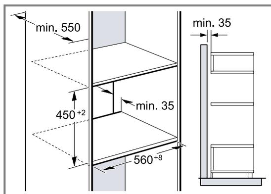
panel or fit a ventilation grille. Ensure that the air exchange is guaranteed in accordance with the diagram.
