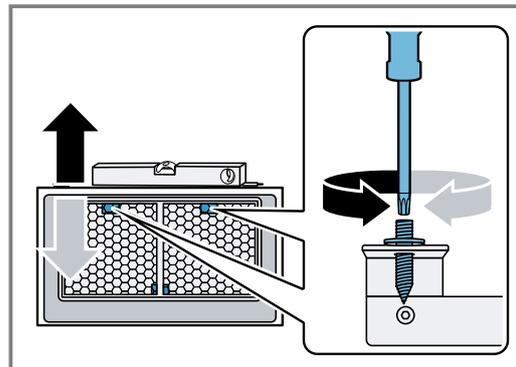
5. Secure the appliance from above using 2 nuts.
