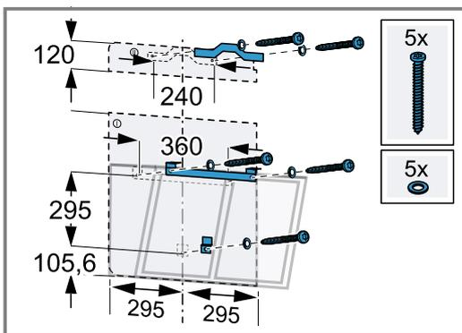
3. Screw the enclosed sleeves fully into the upper appliance bracket.
