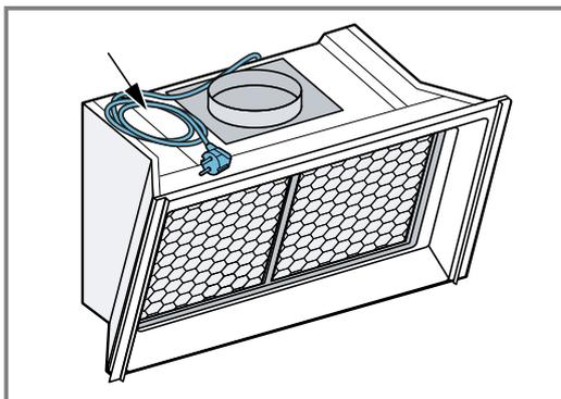
2. Remove the grease filters.
