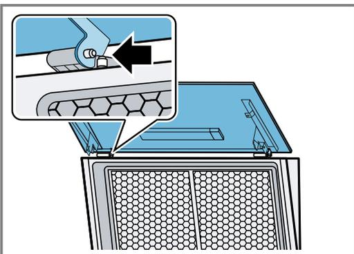
Hold the glass panel firmly until the two hinges are engaged.
