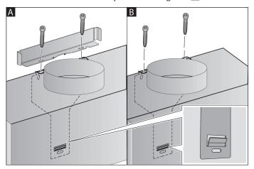
If no duct is to be fitted, screw in the two locking screws without the bracket.
