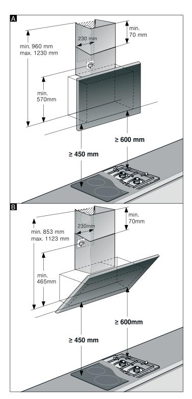
**Note:** We recommend fitting the appliance such that the lower edge of the glass screen is in line with the lower edges of the adjacent wall-hung cabinets. Make sure that the specified safety clearances from the hob are complied with.
