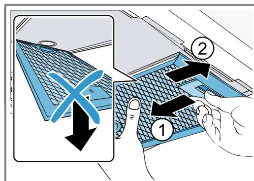
To prevent grease from dripping, hold the grease filters level.
