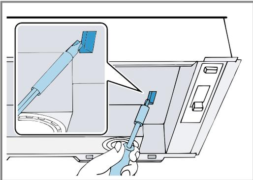
4. Use the enclosed sealing strips to mask the odour filter.
