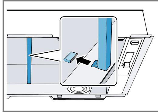
6. Install the grease filters.
