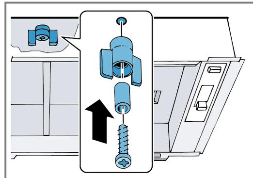
The screw, wing nut and sleeve are included with the odour filter.
