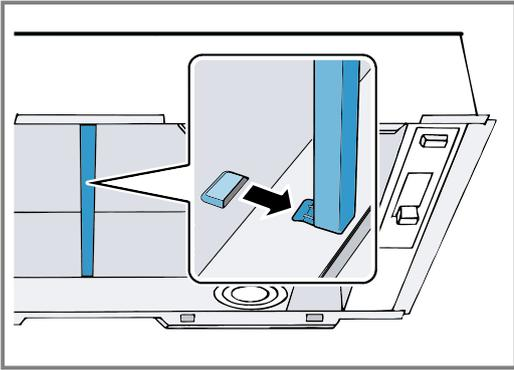
3. Use a screwdriver to push the two tabs on the intermediate floor inwards.
