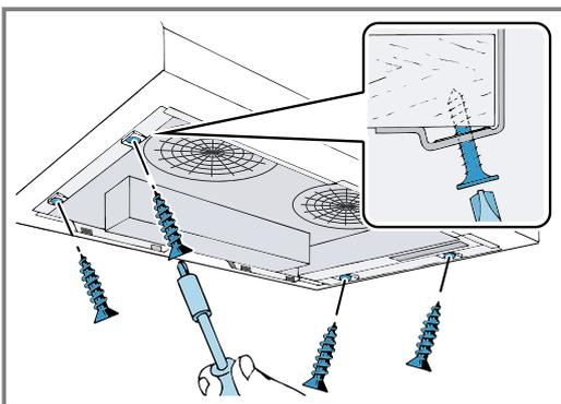
4. Ensure that the lower edge of the appliance is flush with the surround.
