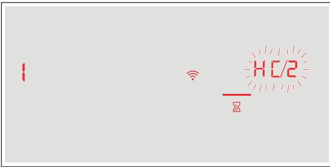
6. Start the app on the mobile device and follow the instructions for manual network registration. The registration procedure has been completed once the **0** value appears on the cooking position display.
