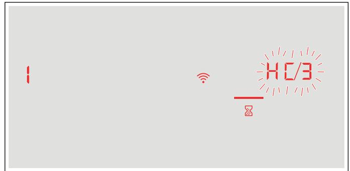
4. Set the **0** value on the control panel. This deactivates Wi-Fi; the
