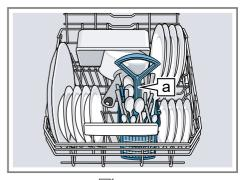
Cutlery basket all Large plates up to a diameter of 31 cm can be arranged in the bottom basket as shown.
