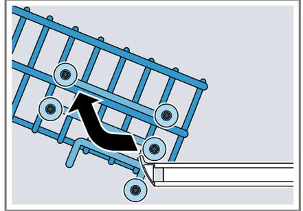
3. Re-attach the basket to the upper rollers (setting 3) or lower rollers (setting 1).
