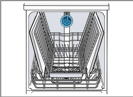
Arrange max. 2 baking sheets and 2 grilles as shown to ensure that the spray jet can reach all parts.
