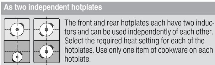
The front and rear hotplates each have two inductors and can be used independently of each other. Select the required heat setting for each of the hotplates. Use only one item of cookware on each hotplate.
