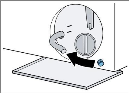
9. Insert the drain hose into the holder.
