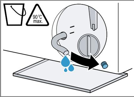
8. Firmly press on the sealing cap.
