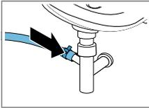
Secure the connection point with a (24–40 mm) hose clamp.
