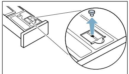
2. Turn the condensation container 180° onto its underside and insert the stopper.
