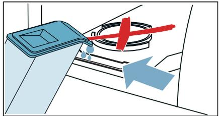
**Note:** If you pour more than 180 ml drinking water into the appliance and **Refresher-container is empty, please re-fill.** does not go out on the display, this means that the drinking water has been poured into the wrong filling hole or the appliance is not fully level. Pour the drinking water into the filling hole on the front or make the appliance level.
