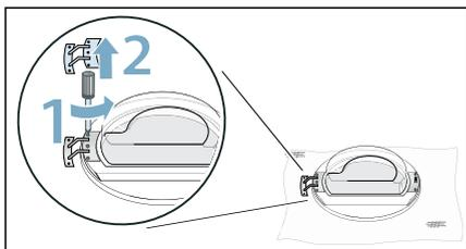
5. Remove the screws from the eyelet and remove the eyelet.
