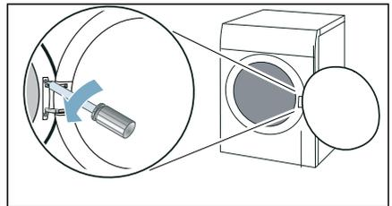
**Note:** Only use a T20 (Torx) screwdriver and no other tools to change the side on which the door is hinged.
