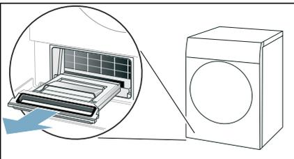
**Note:** The fluff collector may contain fluff and residual water, which may drip out of it when you pull it out.
