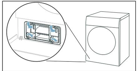
3. Pull the heat exchanger cover out by its grip.
