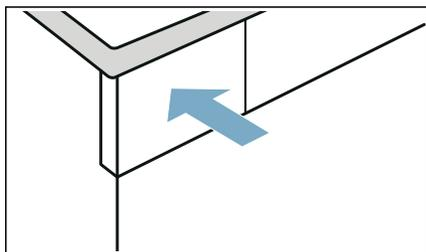
**Note:** The filter in the condensation container filters the condensation water, which is used during the appliance's automatic cleaning cycle. The filter is cleaned by emptying out the condensation water. You should still check the filter regularly for any build-up, and remove this if necessary.
