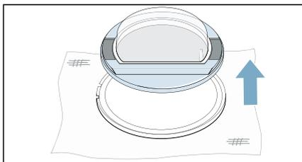
8. Rotate the door ring by 180° and insert the door properly.
