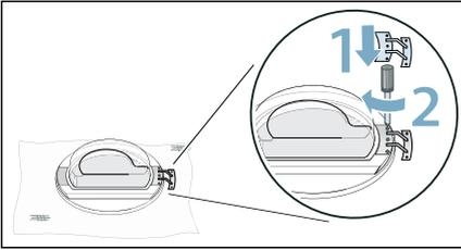
**Note:** Ensure that the door's seal is not jammed or damaged when inserting the hinge.
