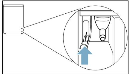
5. Push the drain hose as far as it will go onto the uncovered socket.
