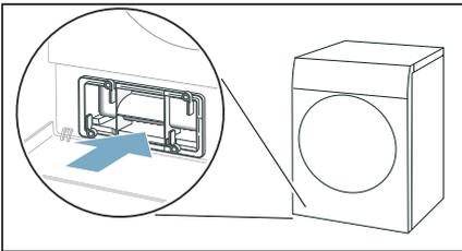
**Note:** You can only slide the heat exchanger cover in if the fluff collector is in the appliance.
