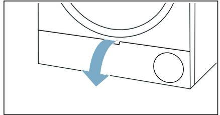
2. Unlock the levers on the heat exchanger cover.
