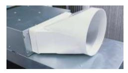
Using a rectangular to round straight adaptor directly on the outlet increases the height needed for install from 207mm to 255mm.
